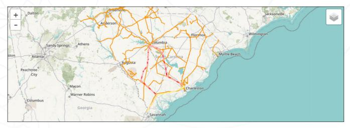
Figure 31: A derailment close to the junction at Yemassee would force a delay and possibly reroute the train. Regional routes are shown for a derailment whose impact lasts from April 26–28 (day 3). Alternate routes (shown in red) are for trains 2 and 3.
