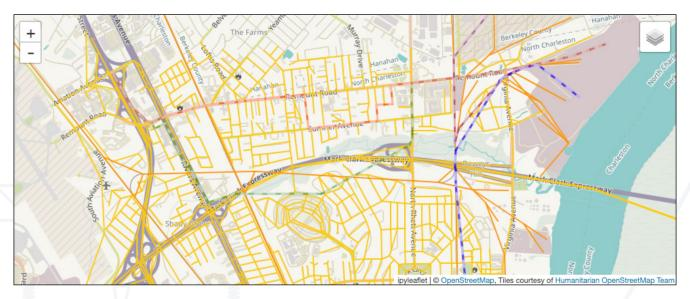
Figure 36: Rerouting road and rail movements in response to a protest on Mark Clark Expressway results in a new potential disruption point at the intersection of Remount Road and Virginia Avenue.
