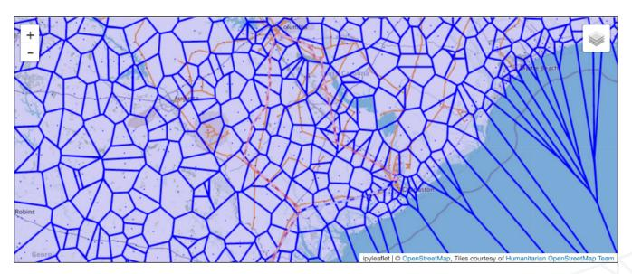
Figure 33: This figure depicts coverage provided by cell phone towers modeled as a Voronoi diagram. The points within each blue region connect to the same (closest) tower. Choice of route taken by rail should also consider the communications networks upon which movements depend.
