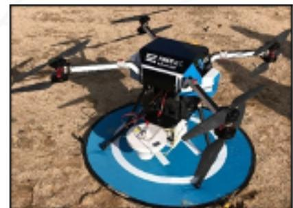
*Figure 4: This AT&T cell on wings, also called a "flying COW," would have been one of the FirstNet-enabled devices provided during the JV 3.0 LFX.*
